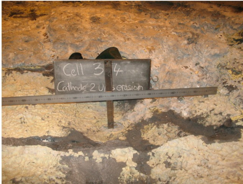
Figure 2. Cathode erosion pattern from a cell autopsy showing the highest erosion occurred in upstream cathode number 2 among the high erosion area between upstream cathodes 1 and 4.
